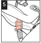
Rebuckle belt. Lap belt portion should now be tight. If not, remove locking clip and repeat all steps.
